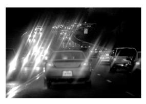
the BGE method described on page 7. Dirt on the windshield also causes glare, as dirt on glass reflects rays of light, either from the sun or headlights.
